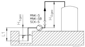
In the case of **emptying waste-water basins** the task of the pump is to convey the medium out of a container which is situated lower than the pump into a collecting container. With the suction line free of medium, the pump must raise the medium by the geodetic suction lift  $H_{S,geo}$ . This is to be differentiated from the length of the immersion pipe L1.
