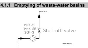
As shown in the diagram, no additional valves are required if it is always ensured that the pump is not siphoned after it is switched off.
