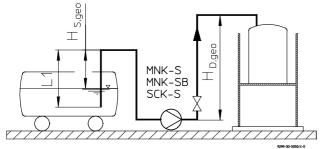
In the case of **emptying with overflow,** e.g. out of a tank truck into an upright tank, the pump has in general a supply, but the medium in this case must overcome the overflow with the geodetic suction lift  $H_{S,geo}$ .
